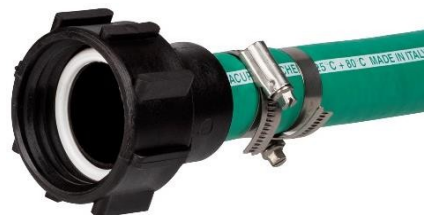
VACUPRESS CHEMI DN25 hose with IBC connector for pallet container (AC-IBF060-H100) in polypropylene mounted with two AISI 316 steel worm bands. White standard LDPE polyethylene gasket visible.
