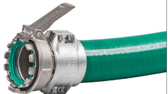
VACUPRESS CHEMI hose DN76 with TANK WAGEN coupling (TW-MK-080-SS) in AISI 316 stainless steel screwed onto an external threaded end (GD-VSLB-080-075-SS) in AISI 316 steel mounted in the hose with an aluminium shell clamp. Green standard hypalon seal (CSM) visible.
