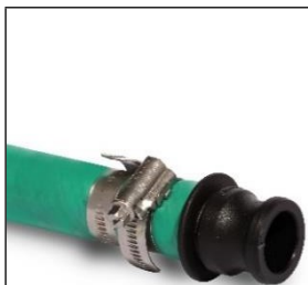
VACUPRESS CHEMI hose DN19 with connector CAMLOCK connector in polypropylene mounted with two worm bands in AISI 316 steel.
